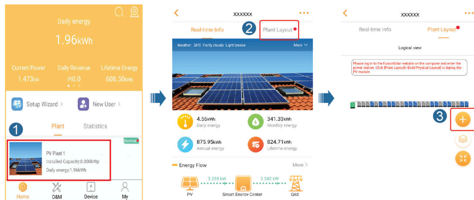
Figure 7-5 Uploading the physical layout template photo (App)
